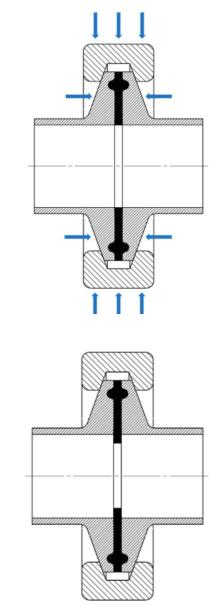
Due to misalignment, we are exposing the gasket to uneven forces. As you can witness in the images the bottom side of the gasket is compressed much more than the top part. This results in a situation where there is gasket material pushed inside the tubing causing a ridge. This ridge has a significant impact on the performance of the whole system. The flow capacity is reduced and the chances of solid material building up on both sides of the gasket are eminent.
