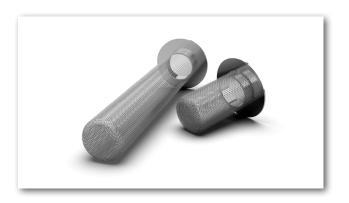
Sock screens are designed to take up a large amount of soil. Flat screens will finally block when too much soil is accumulated. There is also a potential chance that the flat screen can break. Sock screens can take 8 to 10 times more soil and are therefore used in processes where high particle collection is expected. Our sock screens are available in 50 and 150 mm lengths and can be made in a wide range of mesh sizes.
